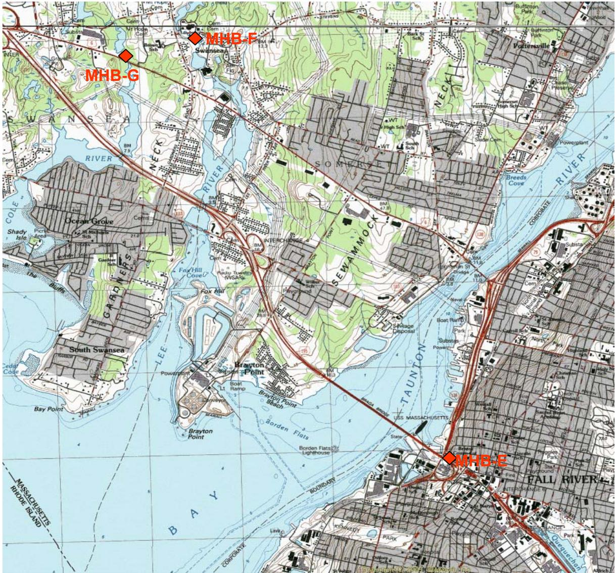
Figure 5. Stream gauging locations on the Quequechan River (MBH-E), Lewins Brook to Lee River (MBH-F, on-going) and Cole Brook to Cole River (MBH-G, on-going). These freshwater inflows transport nutrients to the upper portion of the Mt. Hope Bay basin
